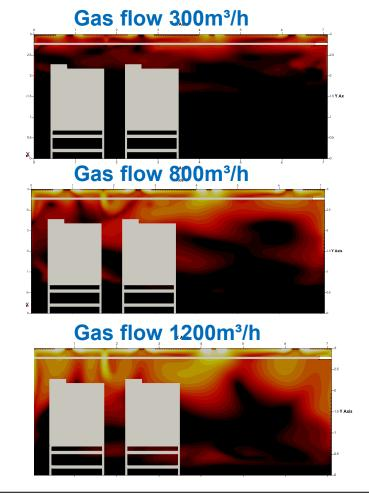
Simulation comparison of a fumigation state – upper representation fumigation isothermal via the ventilation system with swirl outlets – lower image with simple gas injection (300 m<sup>3</sup>/h gas flow) via a pipe piece. The concentration distribution is almost optimal.
